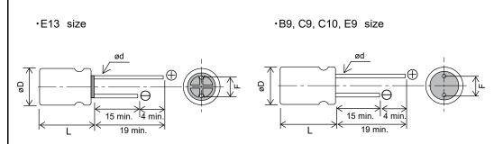
Flat rubber is used for B9, C9, C10, and E9 size.
