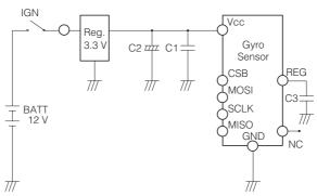
C1 : Design chip capacitor with good high frequency characteristic about 0.1 µF near the terminals of the sensor as possible in parallel as measure for EMS.
