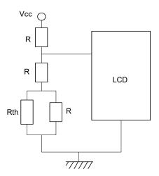
Temperature compensation (RF circuit)
