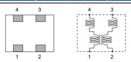
※ The pin numbers shown here are for reference purposes only. Confirm the actual pin number arrangement with the exchanged specification documents.
