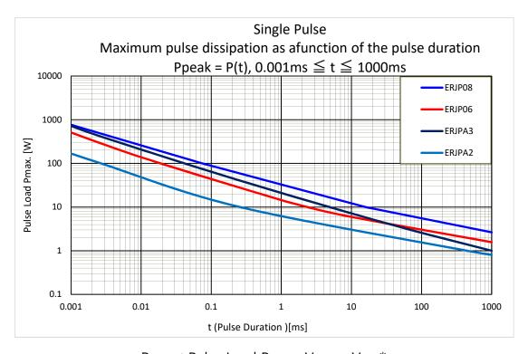
$P_{peak} \leq Pulse~Load~P_{max}~,~~V_{peak} < V_{max}*$   $^*V_{max}$  : Refer to Item of Maximum Overload Voltage in spec sheet.
