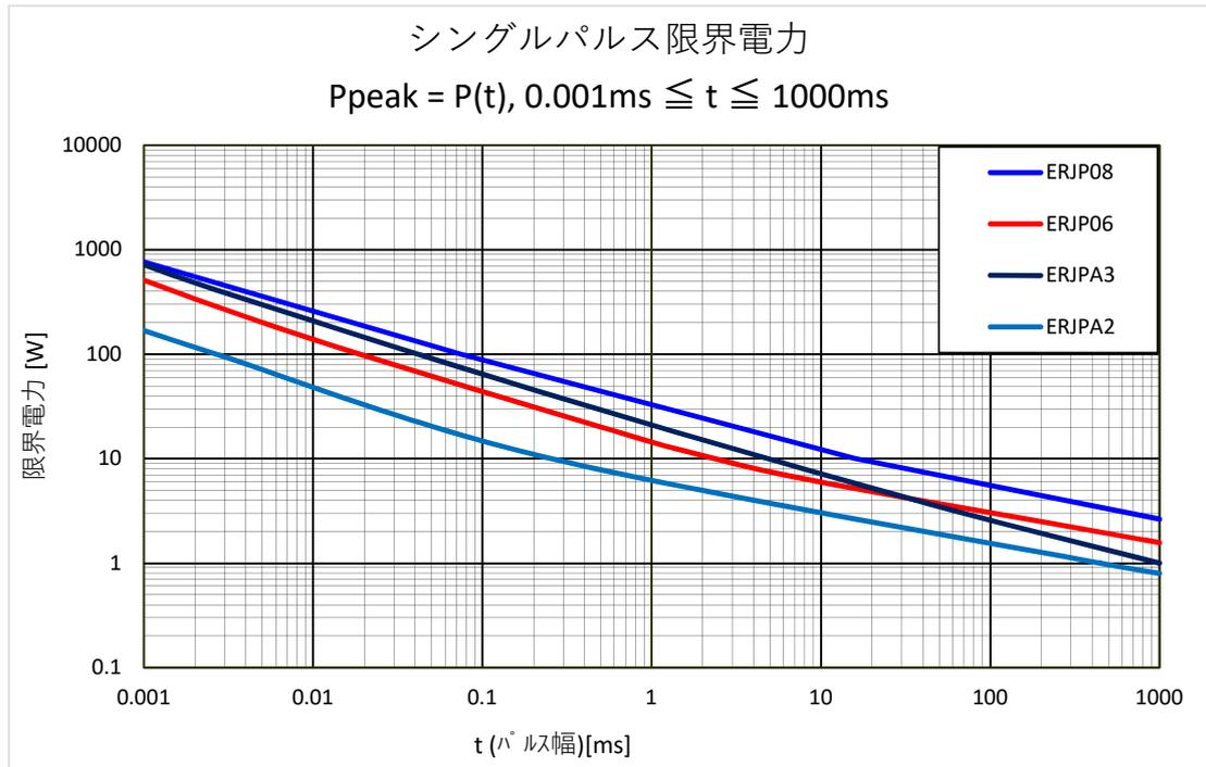
$$P_{\text{peak}} \leq \text{限界電力}, V_{\text{peak}} < V_{\text{max}}^*$$
