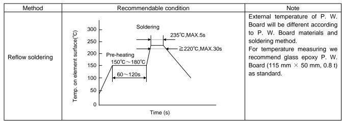
When performing reflow soldering, an appropriate coating thickness of cream solder is 0.10 to 0.15 mm.
