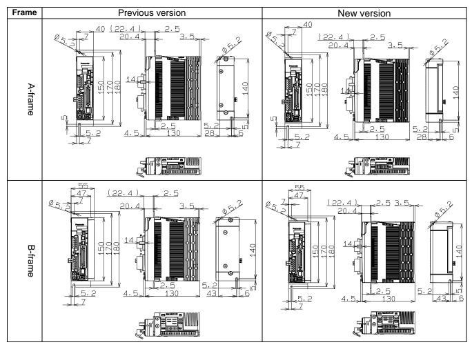
There will be no changes to the characteristics, performance, or dimensions described in the external dimension drawing of the AC servo driver due to this specification change.
