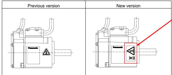
Recycling symbol is added to the high temperature caution mark, and the direction of the high temperature caution label is changed.
