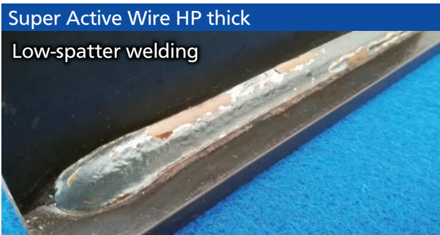
Flat fillet welding YM-50(1.2 dia.), CO 2 ※SUS-MIG: Applicable only to 350 A or less MAG with S-AWP: Applicable only to 350 A or less
